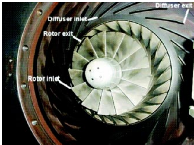
Fig. 9 Components of a centrifugal compressor stage
