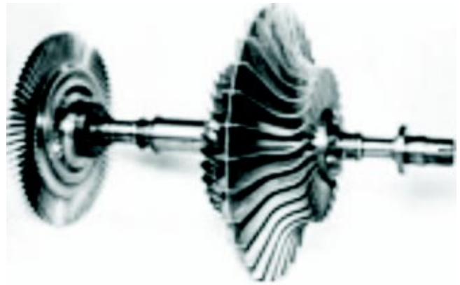
Fig. 6 Rotor assembly of the Whittle's W1 engine
